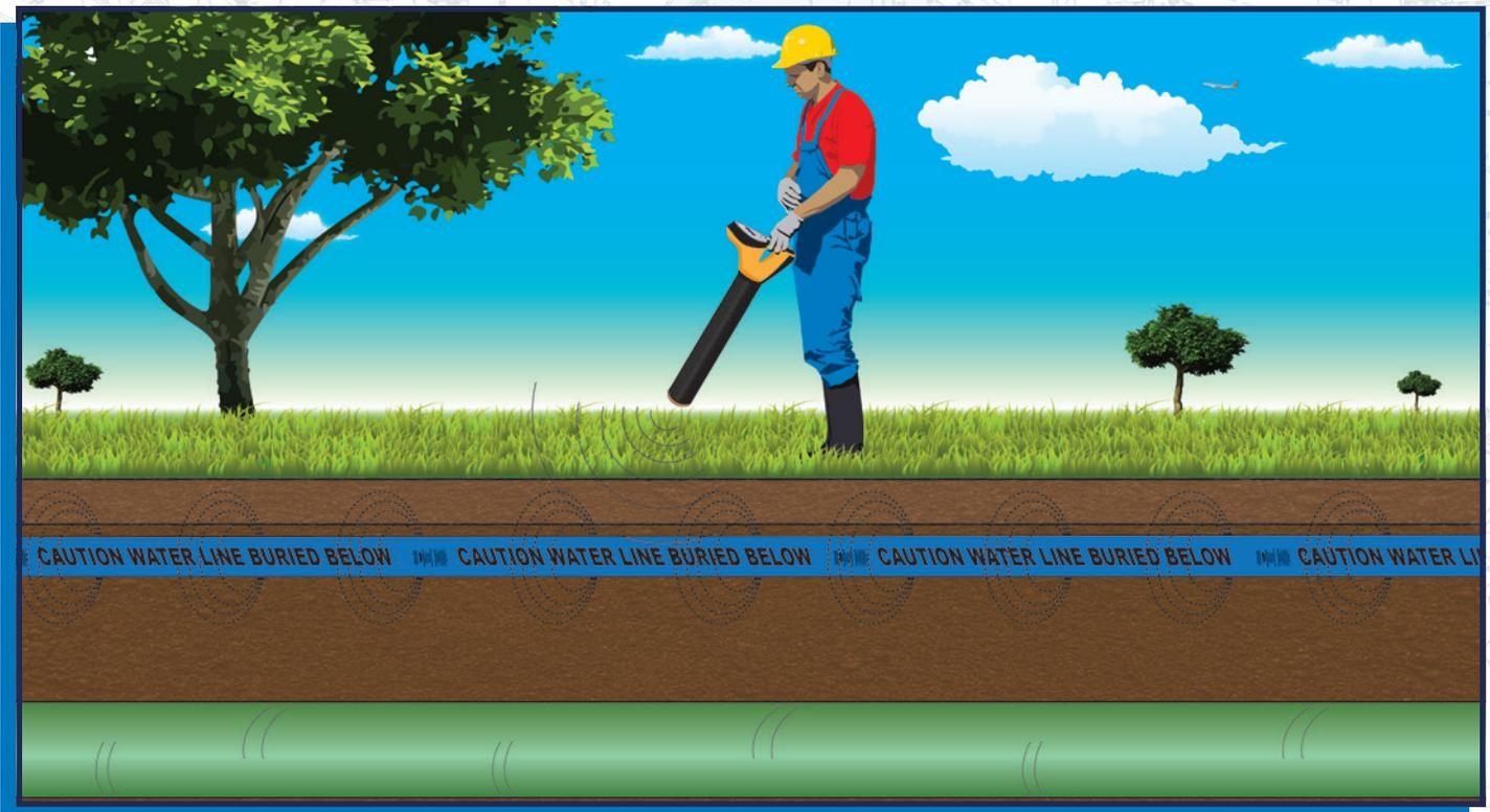
**DESIGNED TO PROTECT, IDENTIFY AND LOCATE UNDERGROUND UTILITY LINES. ALLOWS FOR LOCATION OF THE BURIED UTILITY AND SERVES AS A WARNING BARRIER. CONSISTING OF A LAMINATE COATED SOLID ALUMINUM FOIL CORE AND A CLEAR ENCAPSULATING FILM.**
