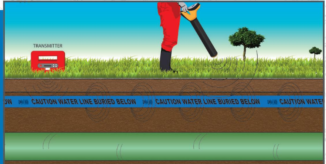
Place the transmitter portion of the locator directly above and parallel to a known section of tape to induce the signal through the ground onto the tape. Alternatively, an inductive couple can be used if a section of the tape is accessible. The transmitter should be in the radio or high frequency mode.
